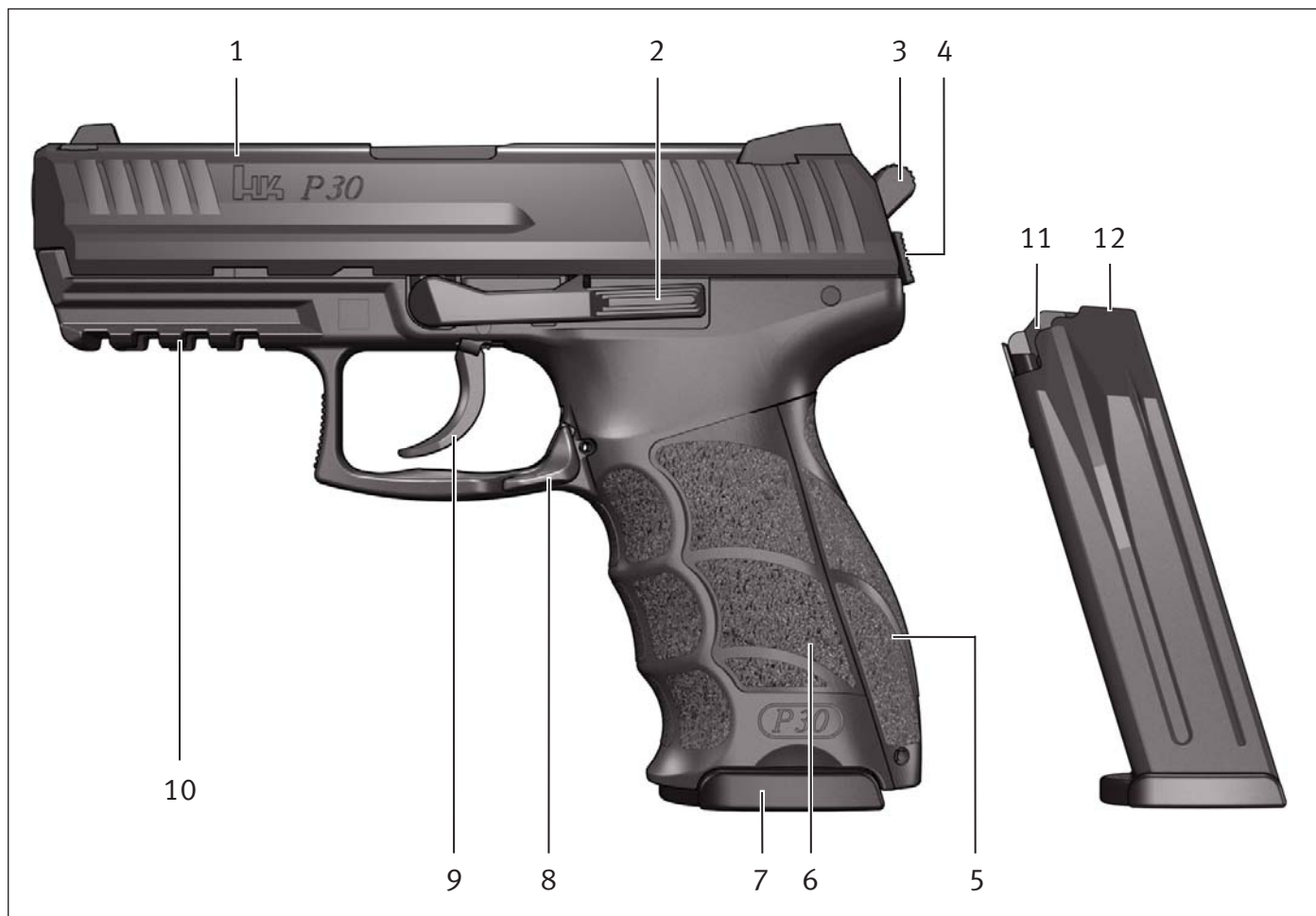
Fig. 1a: P30, left side view
