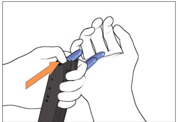
Fig. 38a: Emptying the magazine
