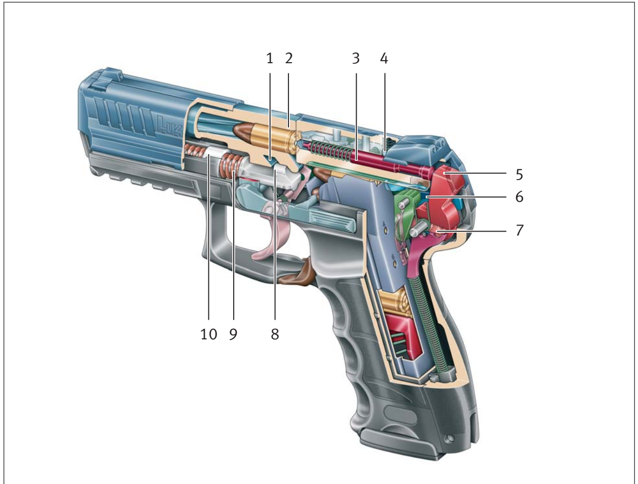
Fig. 13a: CDA trigger variant, cutaway view
